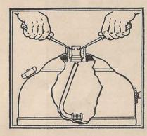
1. Remove Filler Plug to release pressure in fount. Remove burner, unscrew to left. (The Burner will sometimes unscrew at the lock nut connection instead of at the fuel tube. If it does this, unscrew lock nut with pliers and remove handle.
