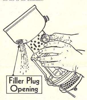
To drain, simply remove Filler Plug and pour gasoline out through Filler Plug opening. The Lantern will light more easily and better with fresh gasoline in the Fount. Whenever available, clean water-white undoped gasoline should be used; however, leaded gasoline and regular motor fuel can be used. CAUTION: Always provide good ventilation—particularly when burning leaded gasoline.
