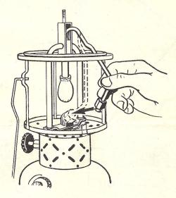
To clean Generator Tip remove Generator Lock Nut and Generator Tube. A cleaning needle is attached to the Wrench which fits into the bottom of the Globe Cage held in place by a Spring. Push Needle through hole in Generator Tip to clean.
