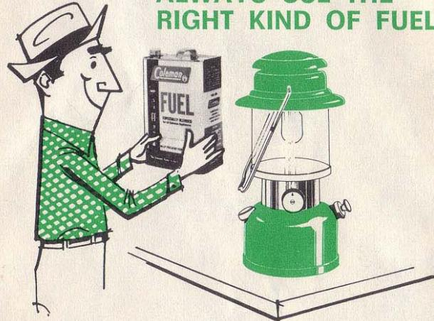
Substances in gasoline which do not vaporize will form carbon in the generator of your lantern. The length of service you get from your lantern and generator depends on the kind of fuel you use. Use only Coleman fuel, or clean "unleaded" gasoline (naphtha). Never use fuels containing lead compounds, or lubricating oils. Store your fuel in a clean, closed metal container.
