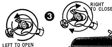
(3) two complete turns to the left. Place thumb over the small hole in handle and pump 35 to 50 full strokes of air into the tank. Then turn pump plunger handle to the right and tighten firmly.
