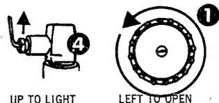
and turn valve wheel (1) wide open to left. Operate burner full open approximately
