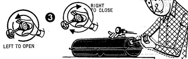
(3) two complete turns to the left. Place thumb over the small hole in handle and pump 35 full strokes of air into the tank. Then turn pump plunger handle to the right and tighten firmly.
