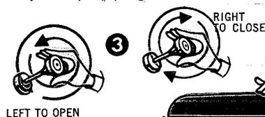
(3) two complete turns to the left. Place thumb over the small hole in handle and pump 35 to 50 full strokes of air into the tank. Then turn pump plunger handle to the right and tighten firmly.
