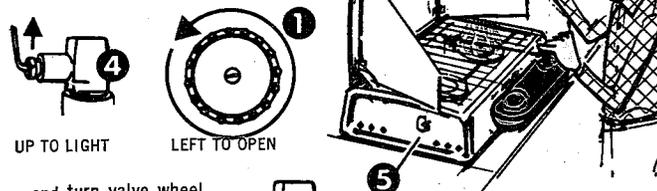
and turn valve wheel (1) wide open to left. Operate burner full open approximately one minute. When flame is quite blue, turn instant-light lever (4) to "DOWN TO BURN" position. Flame can be adjusted by turning valve wheel. Air pressure may be added to tank at any time to give stronger flame. (If flame remains reduced when valve is opened all the way, close and open valve several times. This will clean gas tip.)
