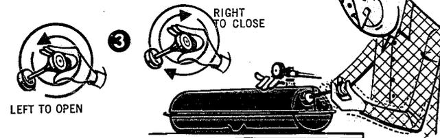
(3) two complete turns to the left. Place thumb over the small hole in handle and pump 35 to 50 full strokes of air into the tank. Then turn pump plunger handle to the right and tighten firmly.
