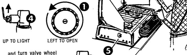
and turn valve wheel (1) wide open to left. Operate burner full open approximately one minute. When flame is quite blue, turn instant-light lever (4) to "DOWN TO BURN" position. Flame can be adjusted by turning valve wheel. Air pressure may be added to tank at any time to give stronger flame. (If flame remains reduced when valve is opened all the way, close and open valve several times. This will clean gas tip.)
