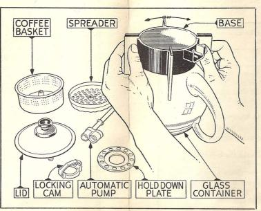
NOTE—Rinse out the GLASS CONTAINER each time before starting the Electro-Brew. DO NOT get the BASE wet as it carries the element. It will not be necessary to remove the Glass Container, for cleaning, oftner than once each month.
