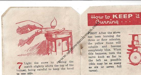
completely blue. When this happens, turn the valve knob as far to the left as possible (this may be as many as six or seven full turns).
